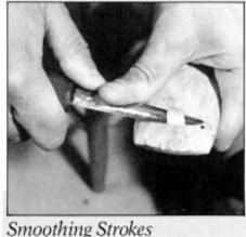
THUMB-PUSH STROKE: Most of the finish work on a spoon can be accomplished with this stroke. Simply rest the knife bevel on the blank and, holding the blank in your other hand, use the thumb of the blank-holding hand to push the blade forward. Use the knife hand to guide the blade at an angle through the stroke for a slicing cut. Aim for increasingly long, smooth strokes as you finish the spoon.
