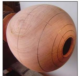
You are now ready to draw the segment lines, but there are some factors to consider. How large is the diameter of the vessel? Typically, 5-6 segments will work well for a vessel approximately 6" in diameter and 7-8 segments for a vessel 8" in diameter.
