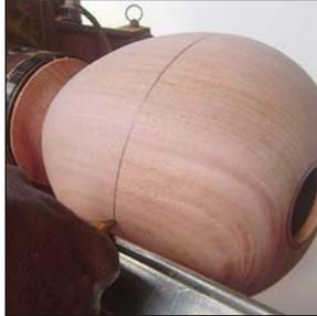
Draw a radial line approximately 1/8" from the edge of the opening at the top. Draw another radial line approximately 1/2" from the bottom.
