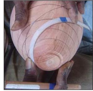
The intersection on the segment and radial lines will be used to draw the spiral lines. You can start the layout on the lathe, but I prefer to do it in my lap. Now it's time to turn off the tenon of the vessel. Continue the segment lines to the base of the vessel.
