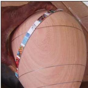
Next, draw the curved portion at the top of the vessel. This will require some trial and error to find the best curve. You will need to draw two lines to determine if you picked the correct curves.
