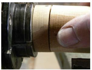
Remove the body from the lathe and attach the lid on to your chuck. You now need to turn the spigot to a depth of 3/32 inches (5 mm) so that you have a tight fit on to the body. (Note the dimple in the end of the spigot). Now this is again where the line you drew on the length comes into play. Line this line up before continuing to the next stage.
