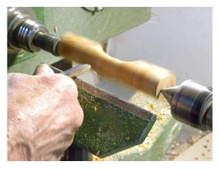
Now taking the piece realign it on the lathe using the offset points start turning from the centre your concave shape you will get a shadow just follow this until you are just half way of the full diameter ie: - 9/16 (15 mm). Once you are satisfied with the shape gently sand and remove any strands from the inside of the opening apply sander sealer to the inside and the curves dry and polish taking care as it is still running out of true. I turn this part at about 1100 revs.
