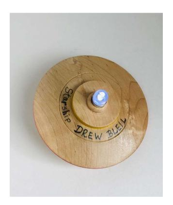
Drill a hole the size of the diameter of the balloon light you are using; the depth should be shallow enough so that the top of the light can be removed to replace the batteries in the future. Use some scrap wood, if necessary, to determine the correct depth. When you are satisfied with the turning and it has the finish completed, epoxy the bottom of the light into the hole.
