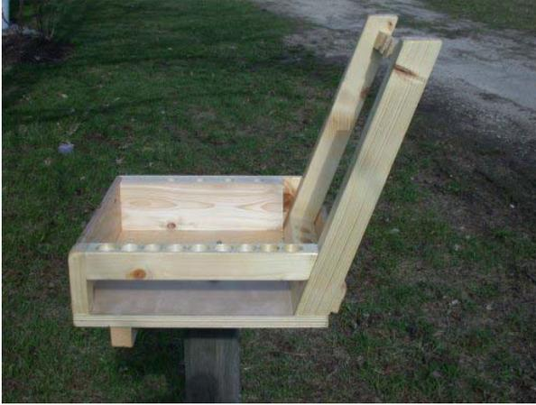
The rear support is tilted back about 15 degrees and the lower portion is dimpled with a Forstner to accommodate the tips of the tool handles.
