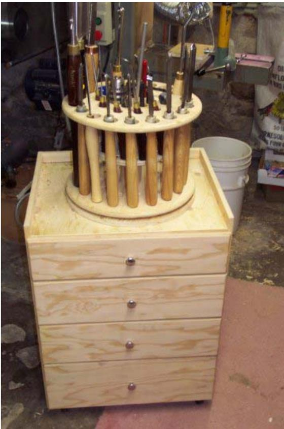
The carousel is 15" in diameter and about 15" high. The top has a ring of 18 holes spaced 20 degrees apart and an inner ring of 11 smaller holes. There are a few  $\frac{3}{8}$ " and  $\frac{1}{2}$ " holes for keys, centers etc. even further in towards the center. It is on a Lazy Susan base and has a mid level support about 8" up from the bottom and about 8" in diameter to support miniature turning tools.
