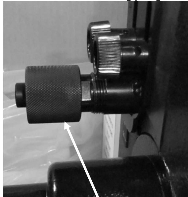
Indexing plunger disengaged
