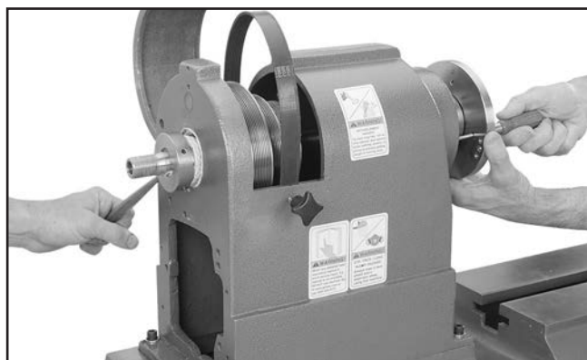
Figure 66. Seating outboard roller bearing.
