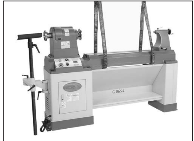
Figure 9. Lifting straps positioned to lift the lathe.
