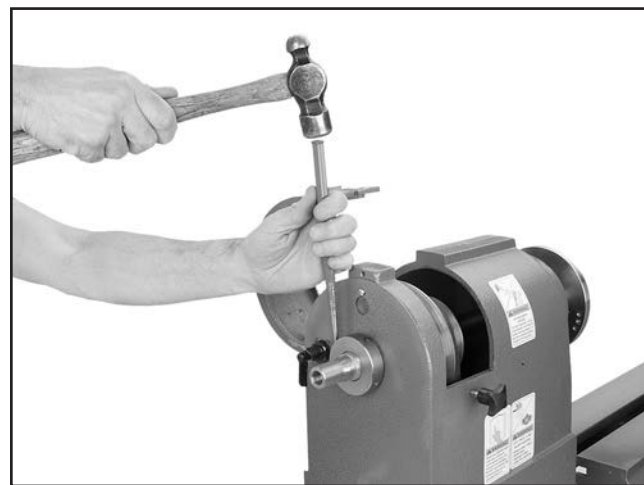
Figure 58. Unseating outboard spanner nut.
