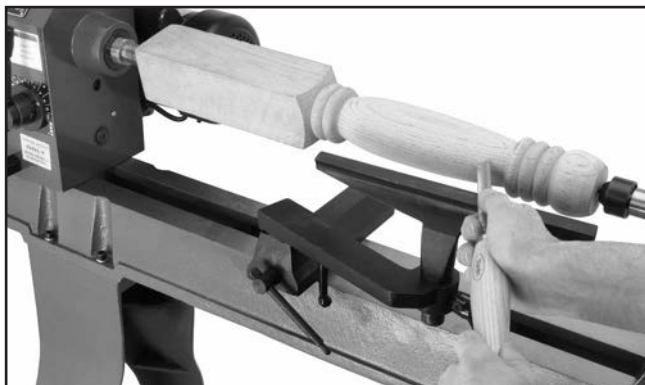
Figure 31. Typical spindle turning operation.
