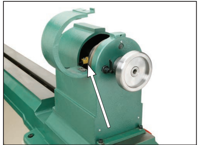
Figure 72. Tachometer sensor location.
