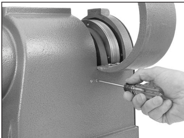
Figure 60. Removing speed sensor screws.
