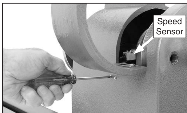
Figure 68. Reinstalling speed sensor.
