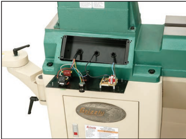
Figure 71. Control panel wiring.
