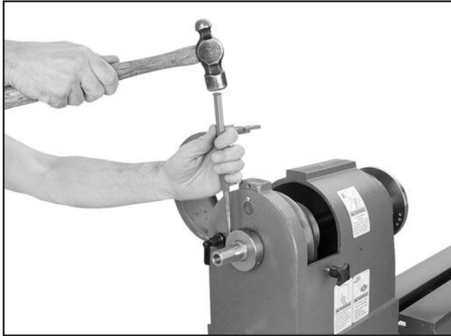
Figure 50. Unseating outboard spanner nut.
