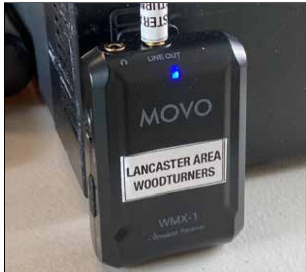
*Movo receiver has a "line out" jack to the computer. The tech monitors mics by plugging earbuds into the headphone jack.*
