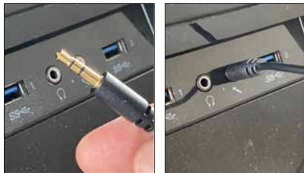
*Movo receiver connects to computer via a TRS plug into the standard mic jack.*
