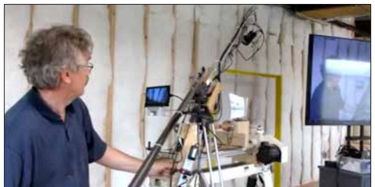
*Doug works the camera boom that usually looks down on the demo lathe. It's wired into the main computer through an HDMI-USB video card. Shopmade boom follows plans published by AAW.*
