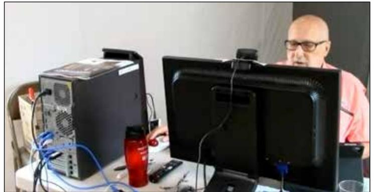
*Lead tech manages cameras and Zoom from our used desktop PC, which connects to the Internet router via wired Ethernet. Zoom image on computer monitor, plus Zoom audio, flow directly to the big TV via 50-foot HDMI cable.*
