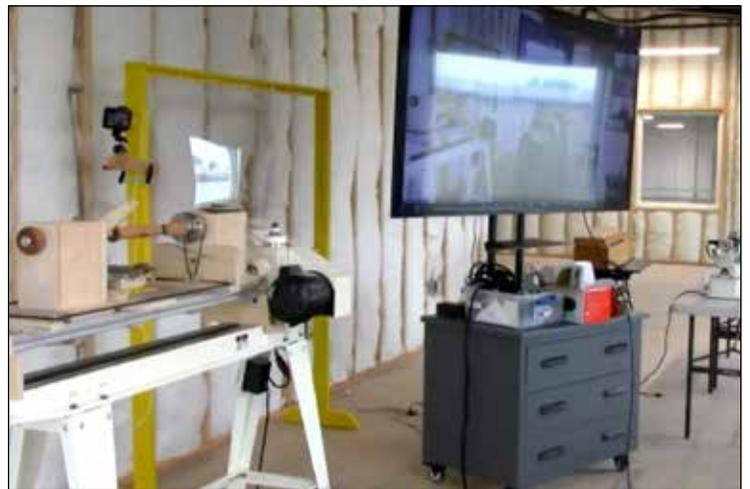
*Tripod camcorder on USB looks at the demo lathe and big TV on sturdy cabinet-stand. WiFi iPhone clamped to yellow safety screen, right rear, sees members in the room. Mixing USB and WiFi cameras is versatile as both can be displayed at the same time.*
