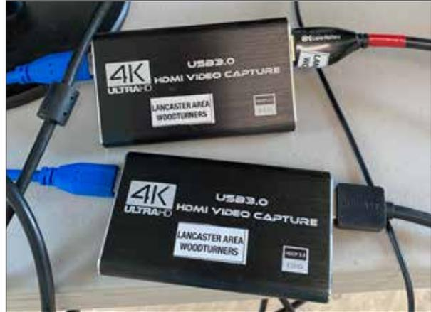
*Video capture cards convert camcorder HDMI output to USB computer input. \$40 cards also have an HDMI-out port for another monitor.*
