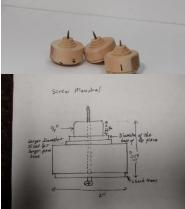
and some epoxy. I follow up with a small hole sized for the screw in the mandrel. I prefer to do the drilling on the lathe but you could do it with a drill press. The little extra weight from the pennies gives the pieces a nice heft. Size the step to match the diameter of the piece you are making so you can easily get it round to your size by turning down to the step. You can add a secondary step for sizing a larger piece. Cutting all blanks to the exact size and add perhaps 1/16''.
