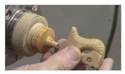
**Finishing:** Traditionally the finish was just a hard wax like carnauba. I was not happy with how just the wax held up with use and prefer lacquer. Seal any dyed pieces with shellac and follow-up with a couple of coats of lacquer. I apply lacquer with a brush on the lathe while turning slowly.
