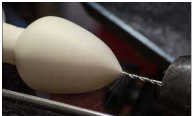
3. Drilling for chain
