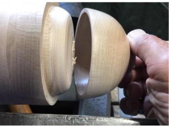
Do you have a snug fit? Use the tail stock to hold it in place and smooth the very top. Drill a hole for the connecting the middle section and the spout (finial). I drilled a one-inch hole.
