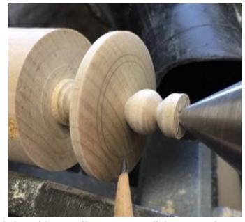
• Before parting off the top of the box from the lathe, with a pencil, put two very light concentric circles on it as guides to locate the eyes and mouth. Also finish the nose.
