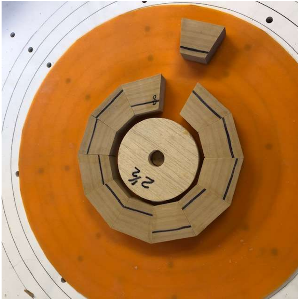
Trial Assembly (dry)
