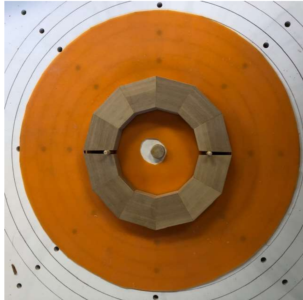
Compensating for poor fit By using spacer rods
